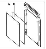
Make sure that you install the middle panel of glass in the seats correctly.
