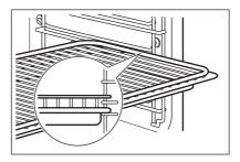
Small indentation at the top increase safety. The indentations are also anti-tip devices. The high rim around the shelf prevents cookware from slipping of the shelf.
